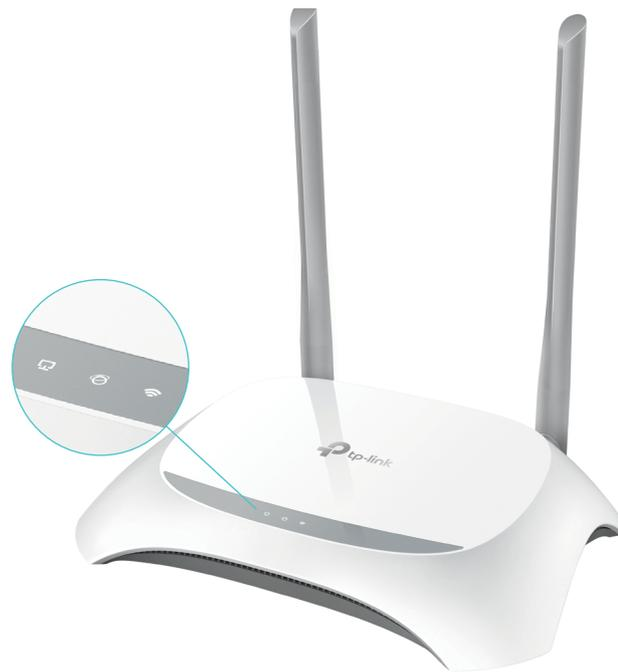
The router's LEDs are located on the front panel. You can check the router's working status by following the LED explanation table.
